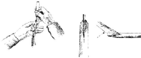
Figure 10: slit the top center of the barrel
